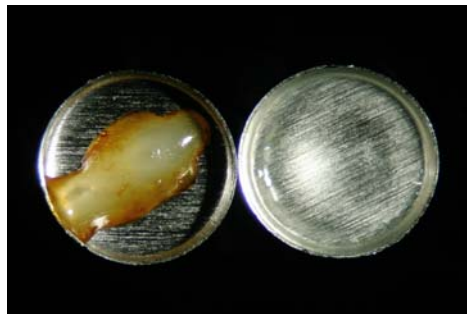
Figure 10, Crosslinking PE (left) shrinks, PP(right) chain scissions and liquifies.
